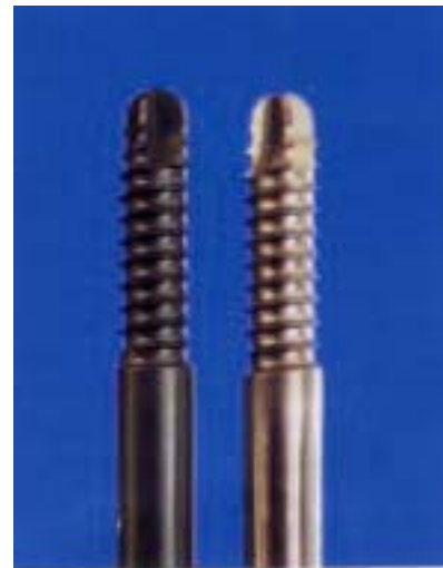
Titanium screws: anodized screw on left
